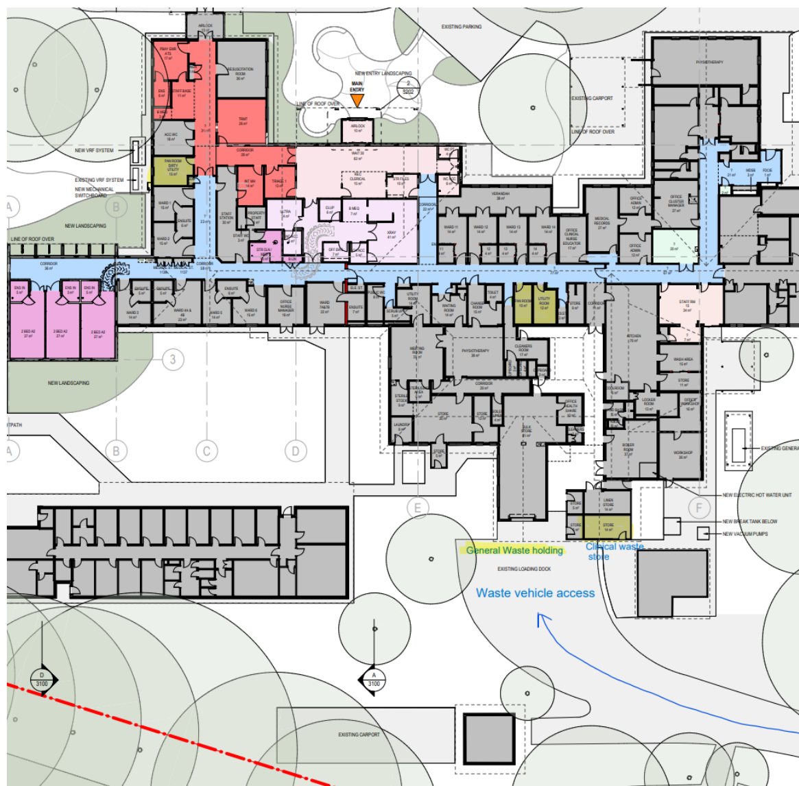
Figure 4: Waste collection points and service vehicle access for management of operational waste
